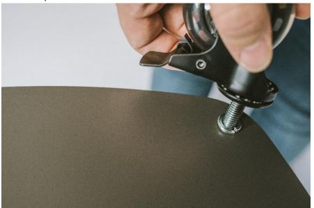
8. Hand tighten wheels using large 15mm Spanner at ¼ of a turn (DO NOT OVER TIGHTEN – WHEEL SHOULD SPIN FREELY)
